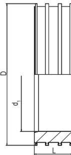
Shaft lining adapter for prefabricated concrete sewage inspection chambers ASF
