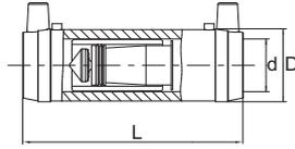
Gas-Stop FRIASTOP with integrated Gas-Stop System by Pipelife
