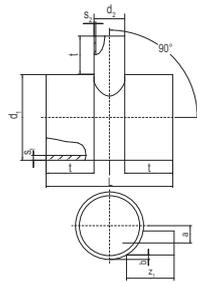
Unequal branch 90° with off-center outlet, SDR 17 (spigot fitting) ATSRS 90
