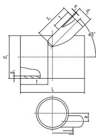
Unequal branch 45° with off-center outlet, SDR 17 (spigot fitting) ATSRS 45
