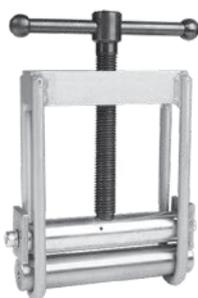
SQM manual squeezing-off tool for the temporary shut-off of HD-PE and PE-Xa pipes d 63 - d 125 in SDR 11 and SDR 17,6.
