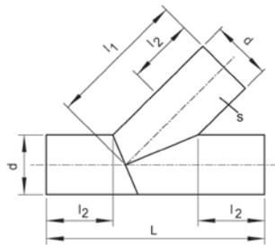
Equal branch with same outlet 45°, SDR 17 (spigot fitting) ATS 45
