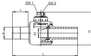
Ball valve for gas KH without flow losses
