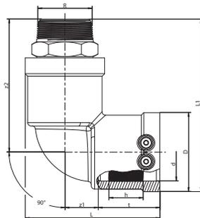
Transition elbow V2A pipe WUN V2A 90
