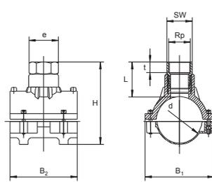
Valve tapping saddle with transition HD-PE/gunmetal VAM RG
