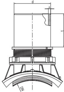
Connecting spigot to clay and concrete pipes ASA MULTI
