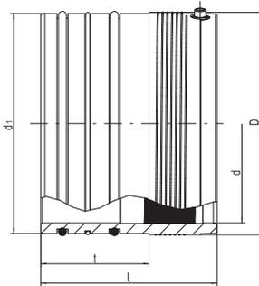
Plug-in coupler for shaft lining adapter AEM
