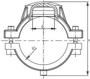
Repair and reinforcement saddle RSV SDR 11
