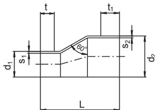
Reducer off-center, SDR 17 (spigot fitting) RES
