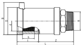
Transition fitting V2A pipe MUN V2A
