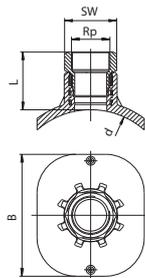
Valve tapping saddle with HD-PE/gunmetal adapter VAM RG TL
