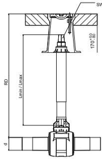
Actuating linkage KBS for ball valves
