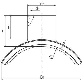
Vacuum-loading spigot saddle SA VL SDR 11 (and SDR 17)
