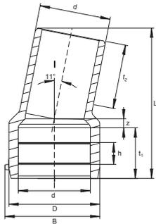
Elbow WS11 SDR 11 with spigot
