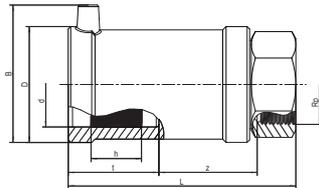
Transition fitting steel pipe USTM
