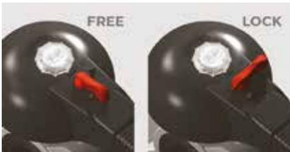
Thanks to the multifunctional handle and the red manoeuvre button on the lever, you can perform a 0°-90° operation and a graduated operation by means of the 10 intermediate positions and a stop lock: the handle can be locked in each of the 10 positions by simply pressing the Free-lock button. A lock can also be installed on the handle to protect the system against tampering.
